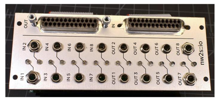
Once those are in place, power up the unit and to make sure no magic smoke escapes. When both the inputs and outputs are left unconnected, the op amps tend to float and may indicate a signal. Don't worry, as soon as you have a snake connected, this will not happen.
